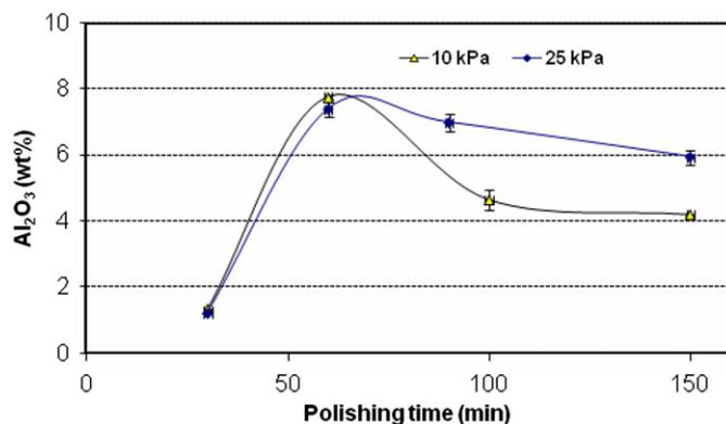
Fig. 7. Variation of aluminum concentration with polishing time.
