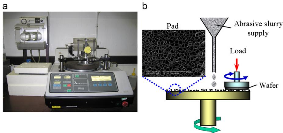
**Fig. 1.** The polishing set-up. (a) The PM5 Auto-Lap Precision Lapping/Polishing Machine used for the polishing experiments in this study; (b) a schematic illustration of a polishing process, showing the porous surface structure of a polishing pad, the slurry application, the polishing loading, and the relative motion mechanism of the polishing operation.
