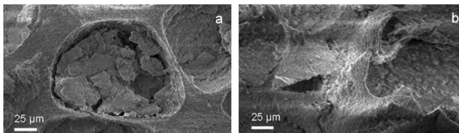
Fig. 8. SEM microphotos of pad after 150 min polishing at pressure (a) 25 kPa, and (b) 10 kPa.
