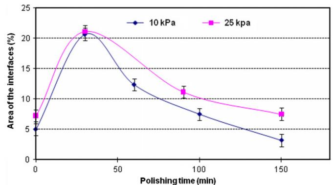
Fig. 6. Contact area variation with polishing time and pressure.
