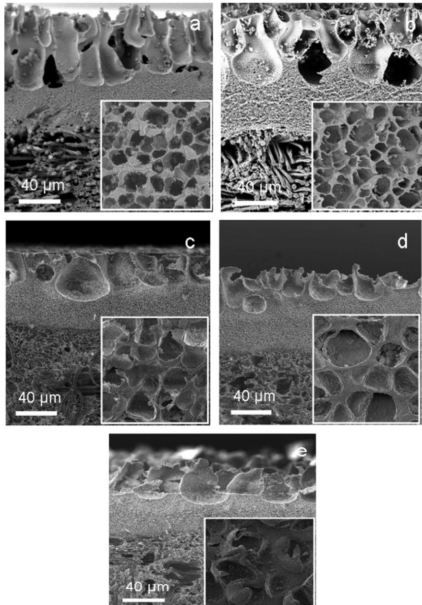
**Fig. 3.** SEM microphotos showing the texture variation of pads with polishing time. All tests were carried out under a constant polishing pressure (10 kPa). (a) new pad, (b) after 30 min of polishing, (c) after 60 min of polishing, (d) after 100 min of polishing, and (e) after 150 min of polishing.
