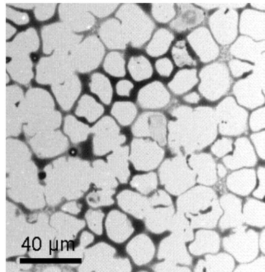
**Fig. 2.** A typical imprint of the contact area between a glass slide and a polishing pad with abrasive particles. The imprint was taken at the pressure of 10 kPa. Note that the dark areas were the contact areas.
