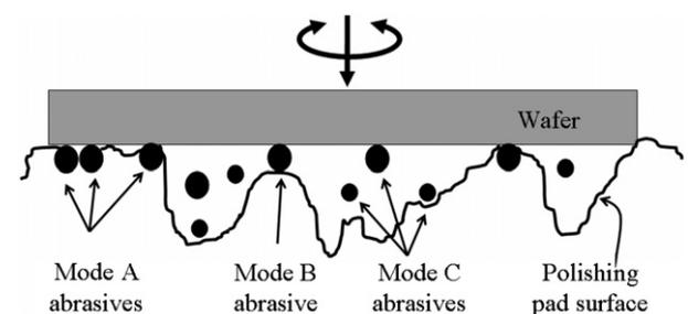
Fig. 9. A schematic illustration of the pad-abrasive-wafer interaction modes.
