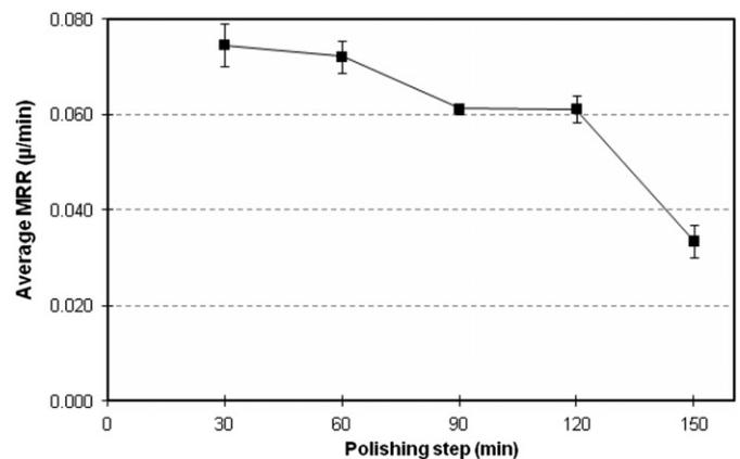
**Fig. 4.** Average material removal rate in thickness of the wafer.
