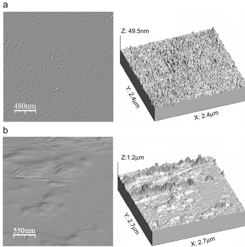
Fig. 5. Polished silicon wafer surfaces. (a) after 30 min of polishing, and (b) after 150 min of polishing.
