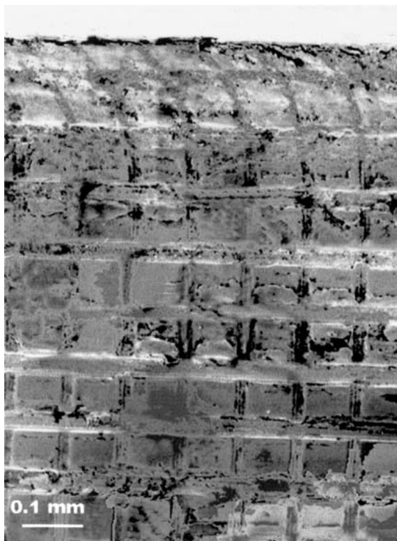
Figure 5 Deformed grid after grinding.
