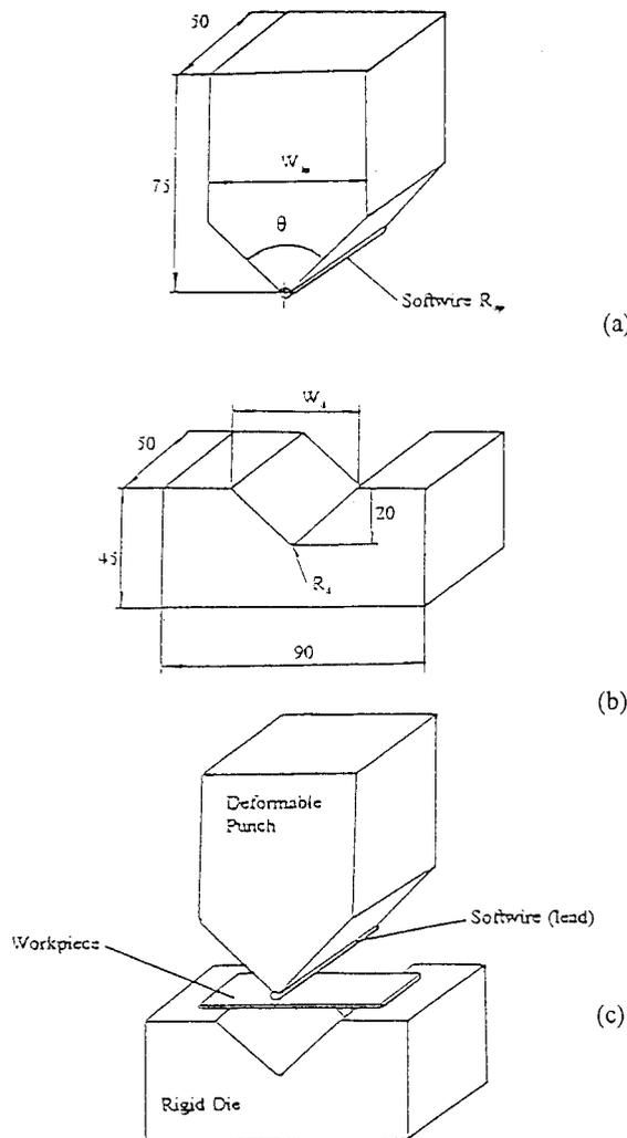
Fig. 1. Geometries for the deformable punch (a) and rigid dies (b); and the tooling set-up (c).
