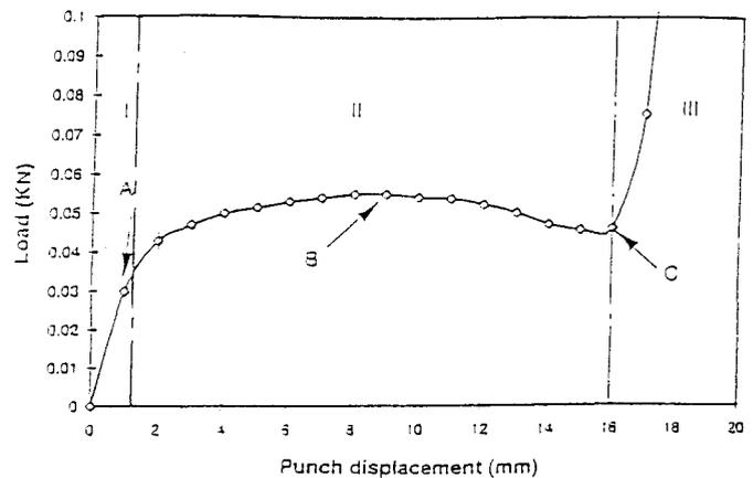
Fig. 4. Three stages of a general load-displacement curve.
