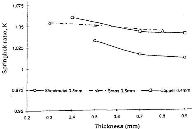
Fig. 9. Effect of thickness on springback ratio  $K$ .
