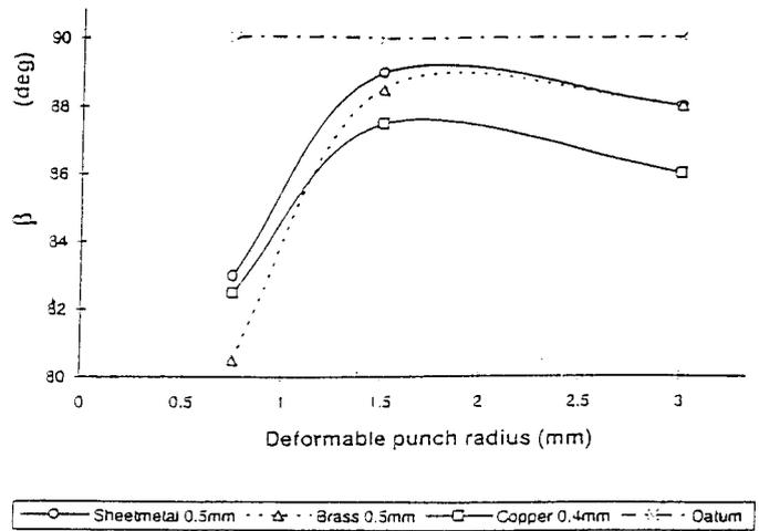
Fig. 6. Influence of deformable punch radius on  $\beta$ :  $\theta=90^\circ$ .
