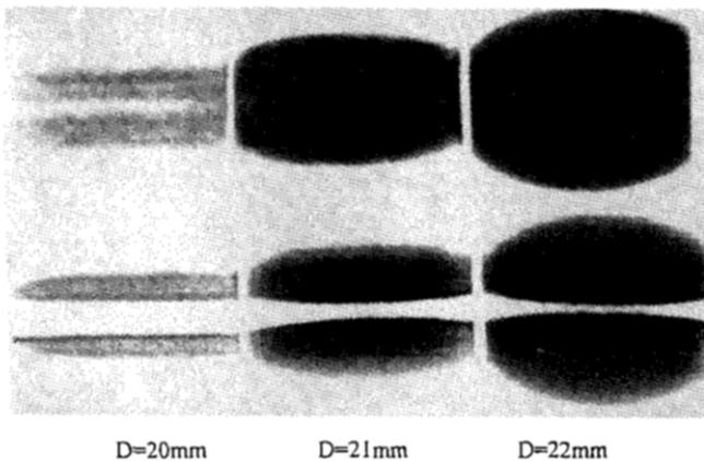
Fig. 11. Impression of contact area obtained from film; top: between lead and specimen; bottom: between specimen and die. D: punch displacement.
