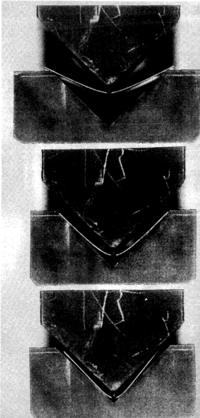
Fig. 3. Photographs of a specimen during test at a displacement of 8, 16 and 18mm, respectively.
