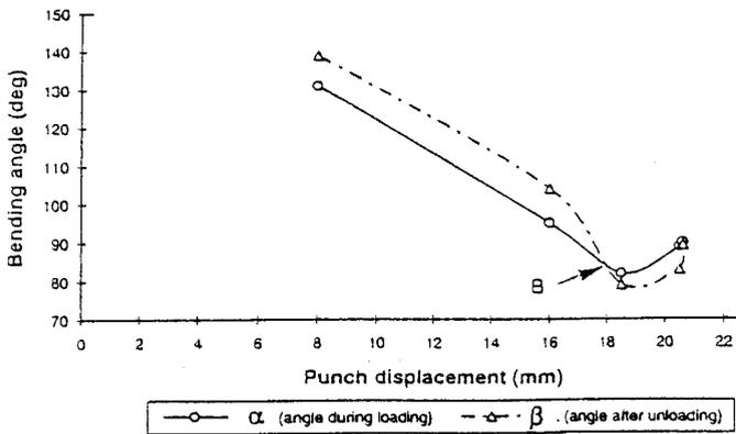
Fig. 5. Angle bent during loading and after unloading: DP90-0.75, RD90-0.75. mild steel,  $t=0.5\text{mm}$ .
