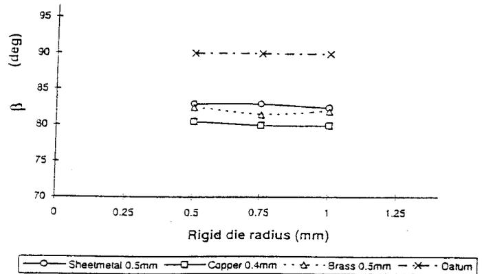
Fig. 7. Effect of rigid die radius on  $\beta$ :  $\theta=90^\circ$ .
