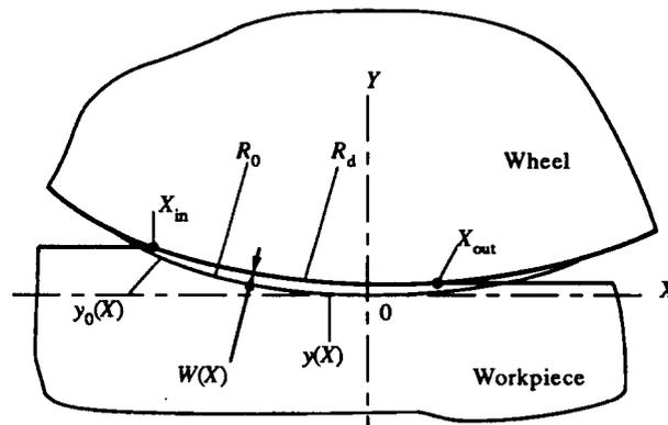
Fig. 1. Interface deformation of a wheel-workpiece system.
