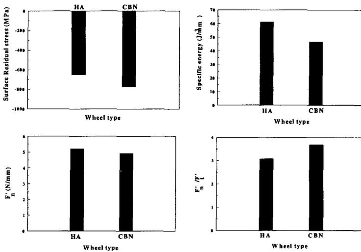
Figure 3. Effect of types of grinding wheels
