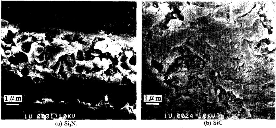
Figure 9. SEM pictures of ground surfaces
