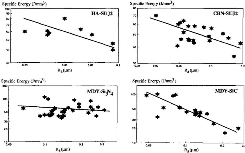
Figure 7. The specific energy and surface roughness
