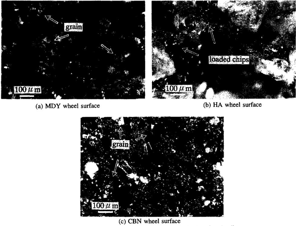
Figure 8. Optical microscopic examination of wheel surface loading
