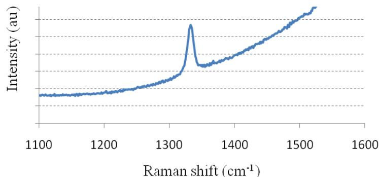
Fig. 3 Macro- Raman (averaging) spectrum of the polished Type 1 PCDC
