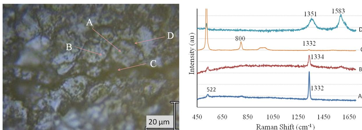
Fig. 4 Polished Type 2 PCDC surface with a crack and the typical Raman spectra.
