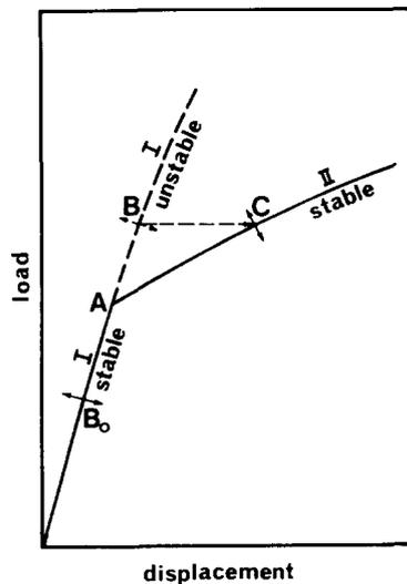
FIG. 1. Bifurcation of equilibrium state of a mechanical system.
