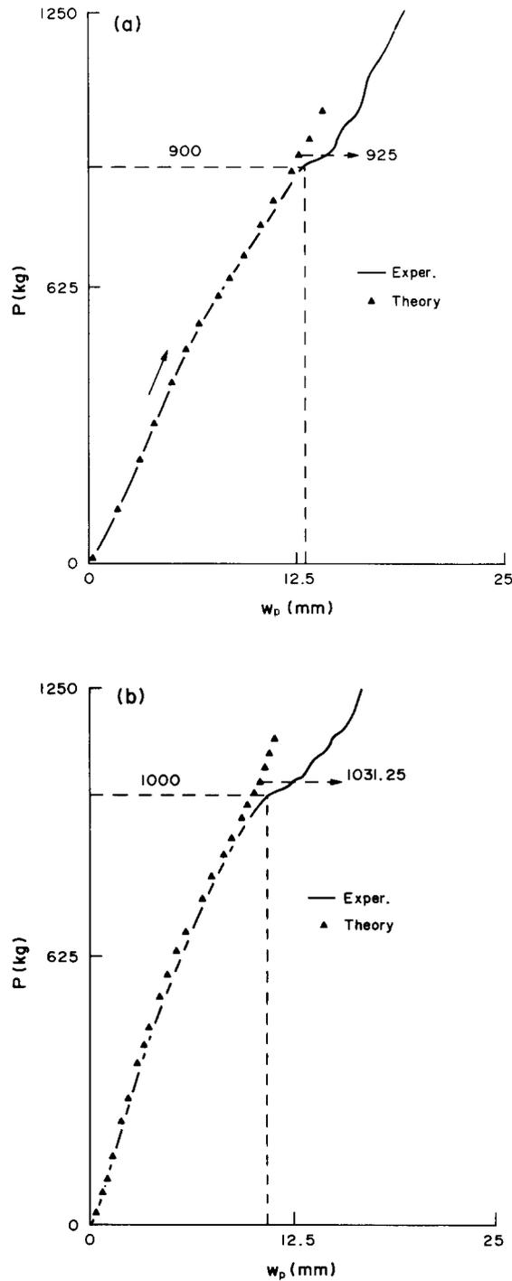
FIG. 3. The external load ( $P$ )–punch displacement ( $w_p$ ) curves: (a) 150-2.0-C45; (b) 150-2.0-C65.
