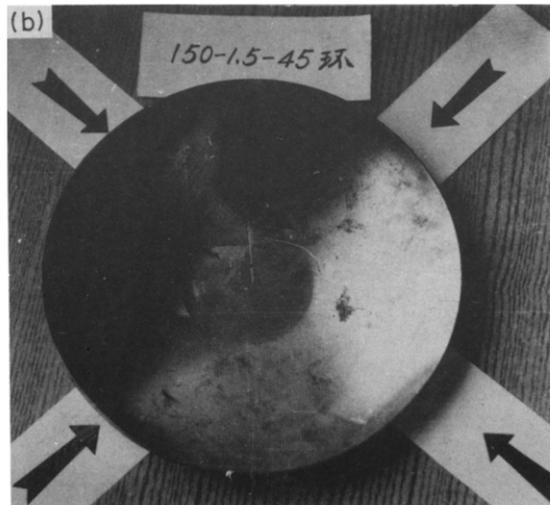
FIG. 4. The wrinkling mode of the workpieces: (a) circumferential shapes of the wrinkling; (b) photograph of 150-1.5-C45 after wrinkling.
