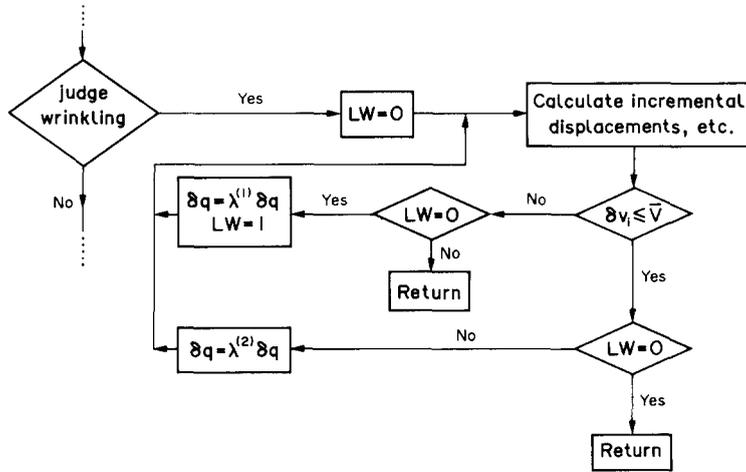
FIG. 2. Flow chart of the algorithm for detecting the plastic wrinkling of the workpieces in the conical cup test.
