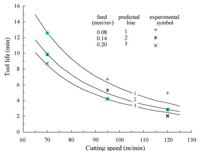
Fig. 5. Variation of tool life with cutting speed and comparison between predicted and experimental results.
