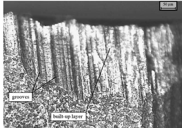
Fig. 1. A typical flank wear scar with grooves and built-up layer.
