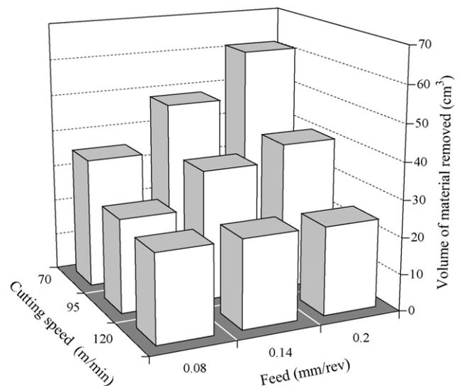
Fig. 3. Variation of the volume of material removal  $W$  with cutting speed and feed.
