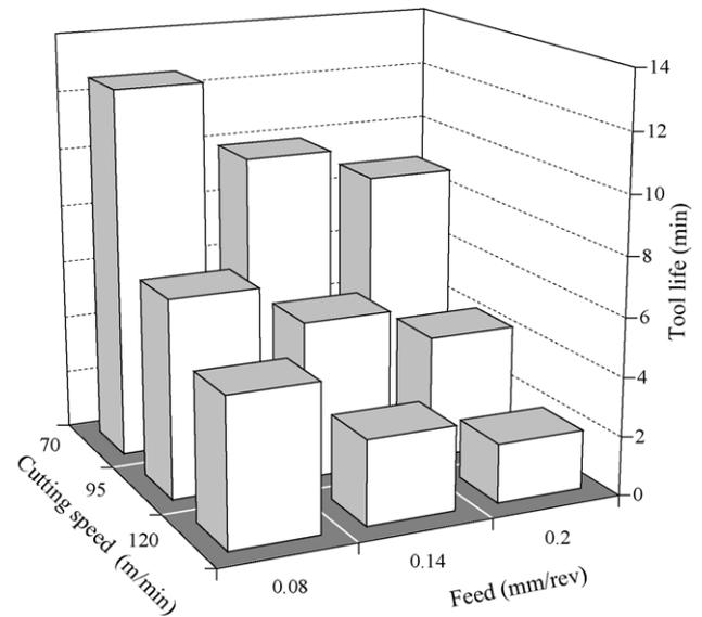
Fig. 2. Variation of tool life with cutting speed and feed.
