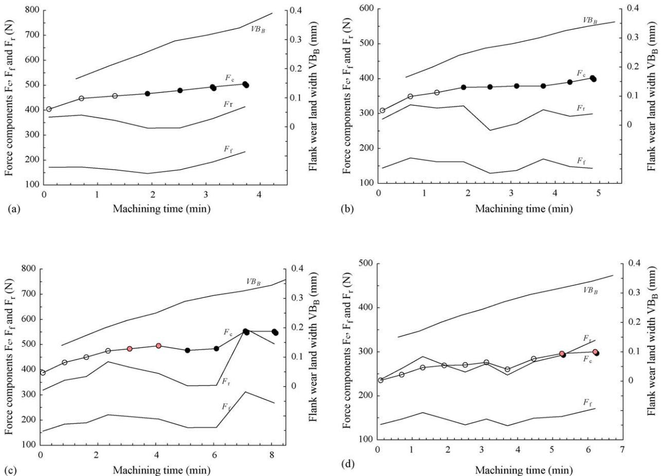
Fig. 4. Variations of flank wear land width  $VB_B$  and force components  $F_c$ ,  $F_f$  and  $F_r$  with machining time: (a) at feed 0.2 mm/rev and cutting speed 95 m/min, (b) at feed 0.14 mm/rev and cutting speed 95 m/min, (c) at feed 0.20 mm/rev and cutting speed 70 m/min and (d) at feed 0.08 mm/rev and cutting speed 95 m/min.
