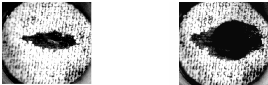
(a) spalling at the chisel edge penetration
