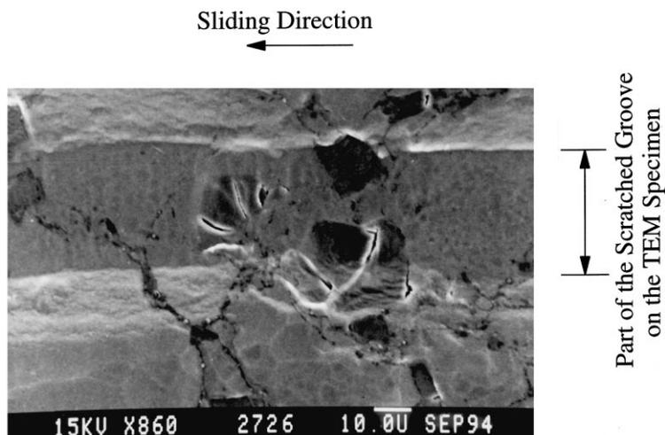
Fig. 2. SEM micrograph showing damage on a scratched groove.
