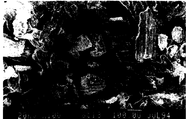
Fig. 7. Typical flaky composite wear debris produced by the mechanism of adhesion.
