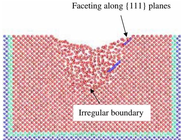
**Figure 5.** The boundary between the amorphous and the crystalline zone.
