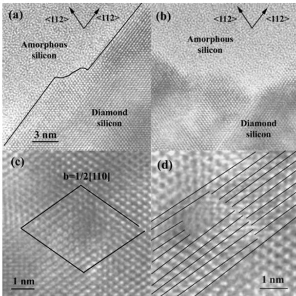
**Figure 3.** HRTEM images from figure 2. (a) Boundary 1–3. Note that the amorphous phase boundary is going along the  $\langle 112 \rangle$  direction and the diamond silicon outside the boundary is almost undisturbed. (b) Boundary 2–4. Note that the amorphous phase boundary does not follow a crystallographic direction. (c), (d) Location ‘4’. Note the dislocation in (c) and the plane shifting in (d) at this location.
