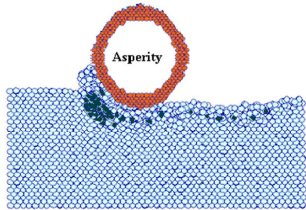
**Figure 4.** Interaction between a moving abrasive and a bulk silicon (darker circles are  $\beta$ -Sn silicon).
