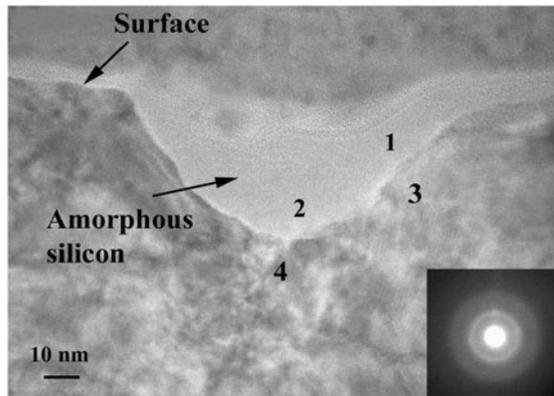
**Figure 2.** The TEM cross-sectional view of a scratch created in the surface modification (the diffraction pattern of the transformation zone is inserted).
