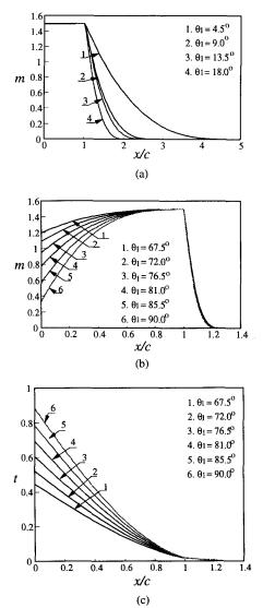
Fig. 5. Distribution of internal forces ( $\mu = 0.05$ ,  $\eta_1 = 50$ , h = 1.0,  $E_s/E_d = 2000$ ,  $E_s/\sigma_r = 1000$ ,  $\sigma_r = 210$  MPa)
