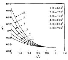
Fig. 4. Variation of springback ratio ( $\mu = 0.05$ ,  $\eta_1 = 50$ , h = 1.0,  $E_d/E_d = 2000$ ,  $E_d/\sigma_y = 1000$ ,  $\sigma_y = 210$  MPa)
