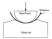
Fig. 1. The schematic of stamping with an elastic die
