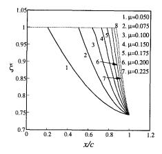
Fig. 6. Effect of friction on the springback ratio ( $\theta_1 = 90^\circ$ ,  $\eta_1 = 50$ , h = 1.0,  $E_s/E_d = 2000$ ,  $E_s/\sigma_y = 1000$ ,  $\sigma_y = 210$  MPa)
