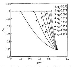
Fig. 7. Effect of elastic modulus of die on the springback ratio ( $\mu = 0.05$ ,  $\theta_1 = 90^\circ$ ,  $\eta_1 = 50$ , h = 1.0,  $E_x/\sigma_y = 1000$ ,  $\sigma_y = 210$  MPa)
