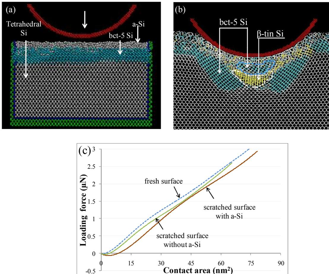
Figure 2: (a) A cross-sectional view of an initial set up for the indentation of silicon with bct-5 silicon in the subsurface, (b) a portion of the scratched surface during indentation, and (c) force-contact area curves of scratched surfaces with and without a-Si (continuous lines) and fresh (broken line) surface on loading.
