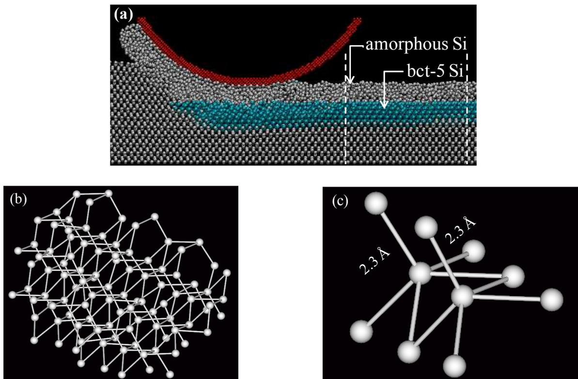
Figure 1: (a) Cross-sectional view of a portion of the scratched surface when scratched along [110] direction, (b) a portion of the bct-5 silicon formed in the sub surface, and (c) structure of the five coordinated atom.
