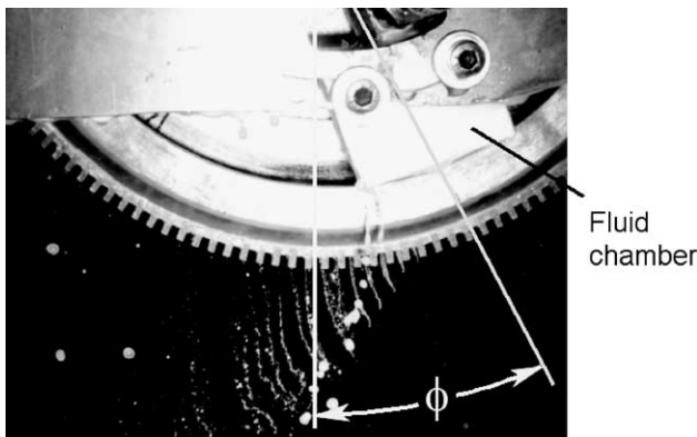
Fig. 3. Flow field of coolant in the forced-flow coolant supply system.
