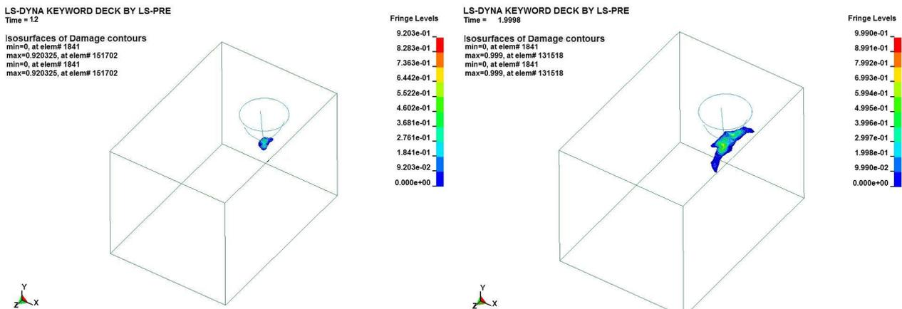
Fig. 4 Isosurfaces of the damage contours, initiation of damage zone in the early stage of the indentation at time  $t = 1.2$ s (left), and propagation of cracks parallel to free surface at  $t = 2$ s (right).
