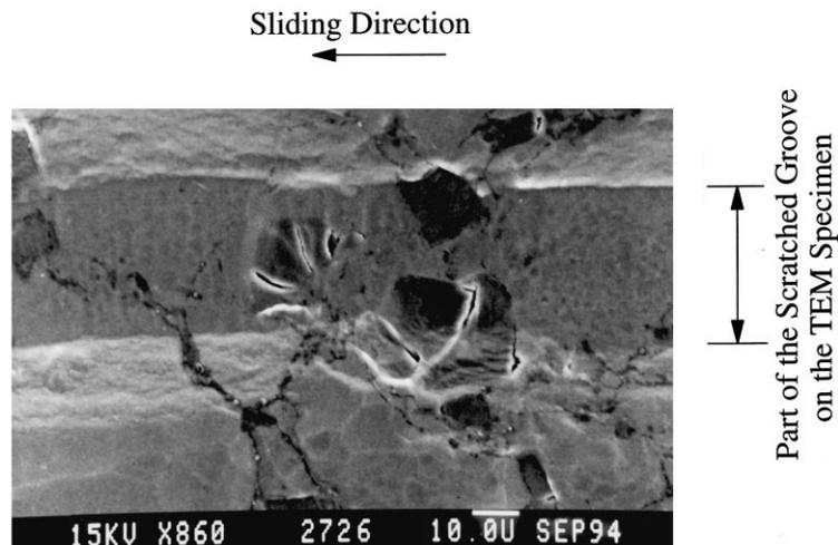
Fig. 2. SEM micrograph showing damage on a scratched groove.
