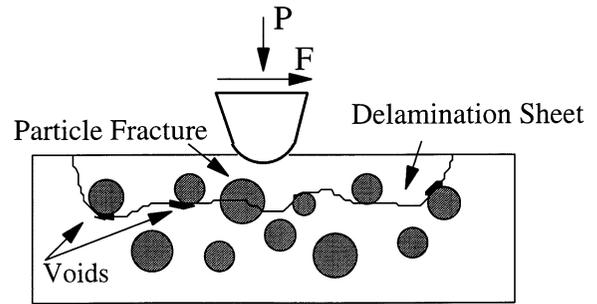
Fig. 3. Illustration of a wear sheet formed by delamination.
