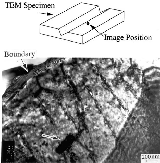
Fig. 4. TEM micrograph of the subsurface structure after scratching showing precipitates and dislocations in a grain.
