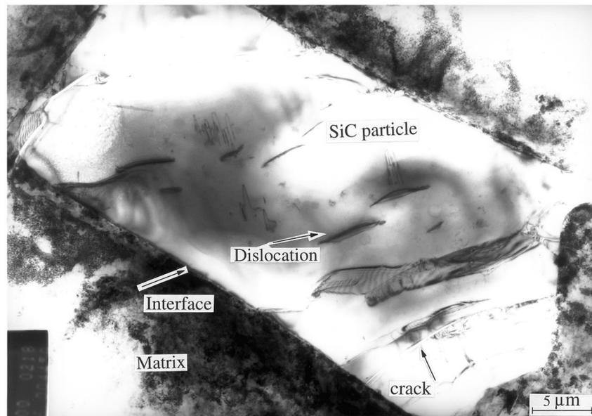
Fig. 5. TEM micrograph showing interface and response of the matrix and a particle by scratching.
