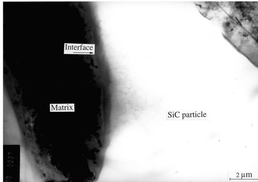
Fig. 6. TEM micrograph showing no dislocation in a particle outside the scratch.
